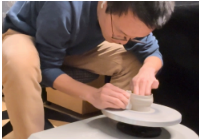
11 Shaping using a physical template. The potter is pressing and trimming the clay.
