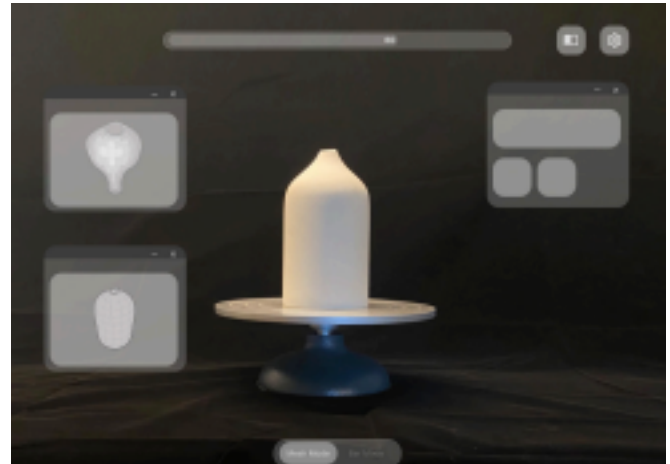
10 Guiding system in improved approach design. The panels are placed on the side to show the 3D model of the intended design on the top, and the reconstructed reality on the bottom.
