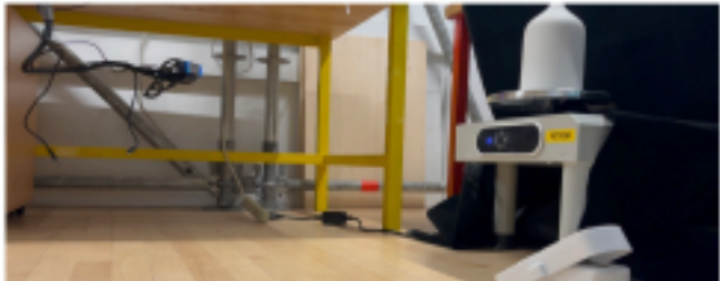
3 Setup in reality. Only side camera used to capture elevation view of the pottery with black drop cloth as background.
